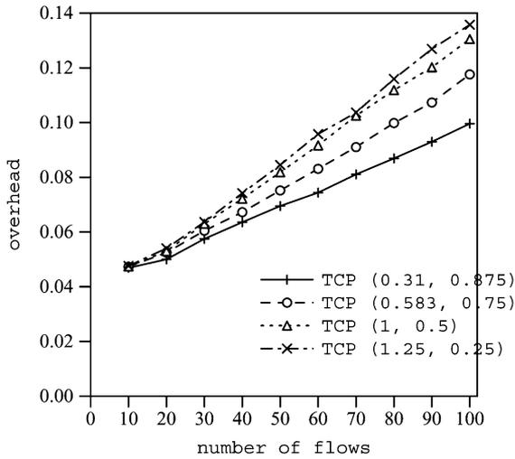
Fig. 4. Overhead over wired network (10 Mb/s bottleneck link).
