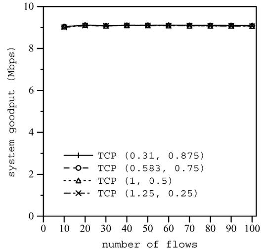
Fig. 2. Goodput over wired network (100 Mb/s bottleneck link).
