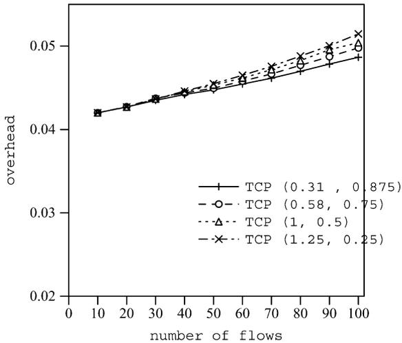
Fig. 5. Overhead over wired network (100 Mb/s bottleneck link).
