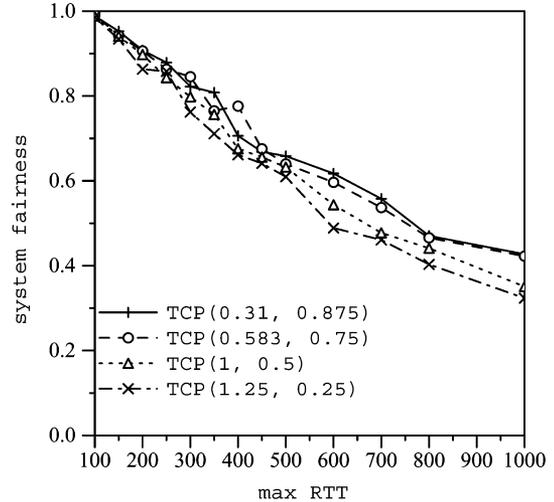
Fig. 16. Fairness with drop-tail gateway (10 Mb/s bottleneck and 20 flows with diverse RFFs).
