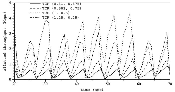
Fig. 13. Allotted throughput with 500 ms handoff (one flow).
