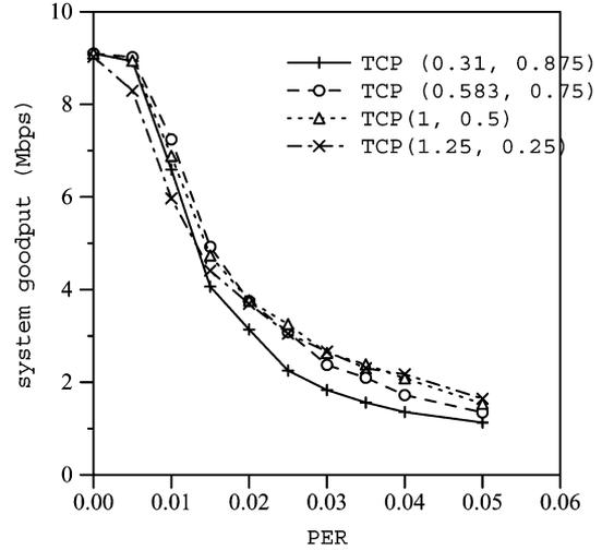
Fig. 9. Goodput over heterogeneous network (ten flows, 10 Mb/s bottleneck).
