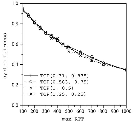
Fig. 17. Fairness with RED gateway (10 Mb/s bottleneck and 20 flows with diverse RTTs).
