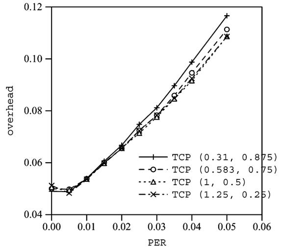
Fig. 12. Overhead over heterogeneous network (100 flows, 100 Mb/s bottleneck, and 10 Mb/s wireless link).
