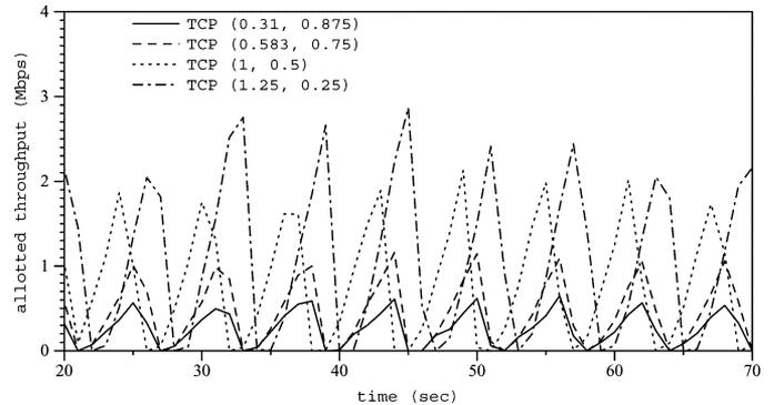
Fig. 14. Allotted throughput with 1 s handoff (one flow).
