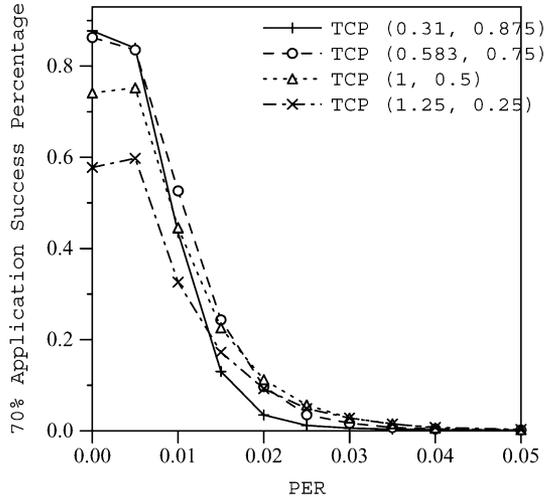
Fig. 15. 70% application success percentage (100 flows, 100 Mb/s bottleneck, and 10 Mb/s wireless link).
