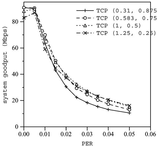
Fig. 10. Goodput over heterogeneous network (100 flows, 100 Mb/s bottleneck, and 100 Mb/s wireless link).
