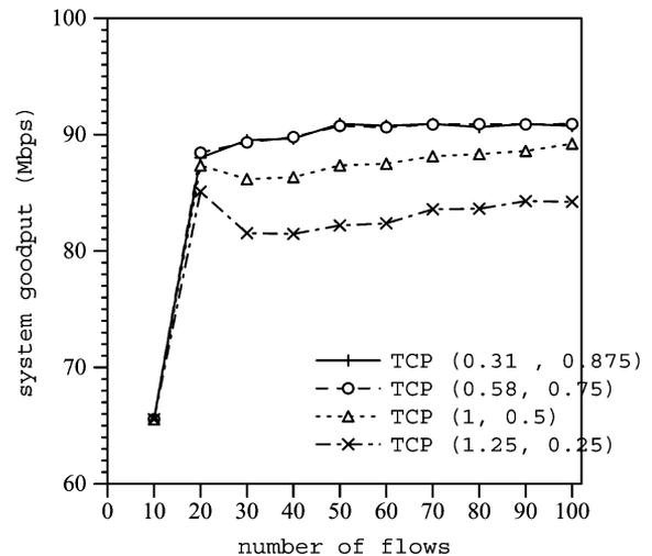
Fig. 3. Goodput over wired network (100 Mb/s bottleneck link).
